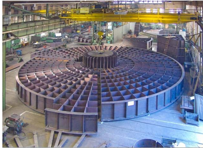
Regenerative Heat Exchangers with Rotating Heating Surfaces (ROTHEMÜHLE-Rotor System, first described by Fredrik Ljungström)
